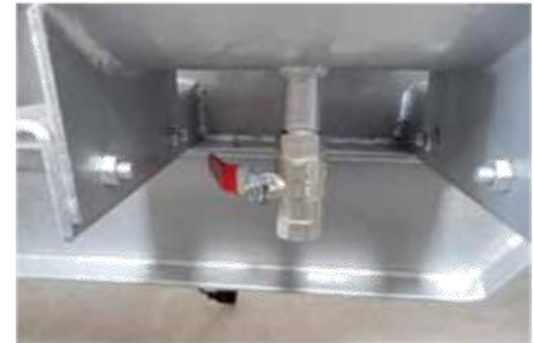
6- Air tank. It should be open (In the sample it looks closed) after finishing the discharging for 10 - 15 seconds for oil discharging.
