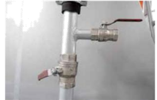
9- It will be used to discharge the air in the tank. Up handle is helping to discharge the air, Below Handle is another jet valve for discharging the cement.
