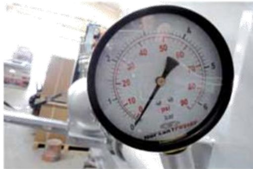
11- It must be between 1 - 2 bar. When the discharge ends, it will show 0.
