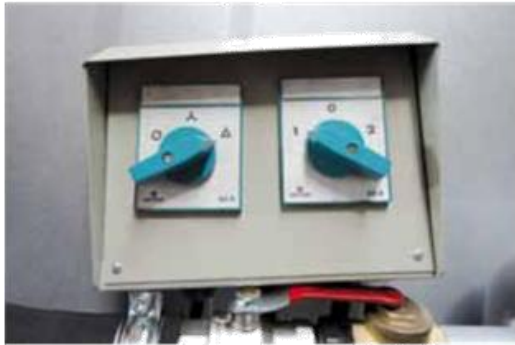
1- Left button for self starter, Right button should be on 1 or 2 according to the direction on image 2.
